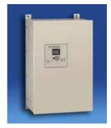
The F7/Configured package provides an F7 in a NEMA 12 FVFF or NEMA type12 enclosure, with space for several commonly used options, such as reactors, RFI filters, circuit breakers, etc. The F7/Configured has been designed for flexibility in providing the features and options commonly demanded by industrial control designers.
